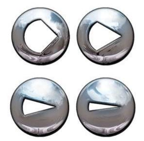
a small angle opening, such as a 15° ball, furnish a linear inherent flow characteristic. medium angle V-Port valves such as a 30° ball furnish a modified equal percentage inherent flow characteristic. Custom ports are also available to meet special control requirements. designed with flexibility in process conditions in mind, the Cv and control characteristics are easily changed by simply changing the ball.
